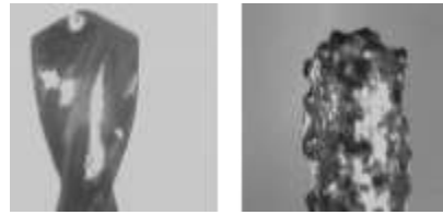
Figure 6: (Left) 0.3 mm cemented carbide micro-drill wear. (Right) 0.6 mm diamond micro-drill wear
